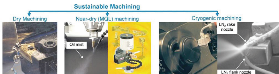
Figure 1.1 Sustainable machining options as machining with dry, MQL, cryogenic cooling (Jawahir et al. 2016).
