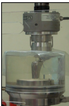
Figure 2: Complete assembly before starting test in INSTRON 8872 machine.
