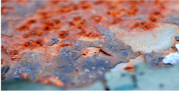
Figure 5: Pitting in Centurion.
