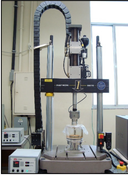
Figure 6: Test assembly after 10^6 cycles.
