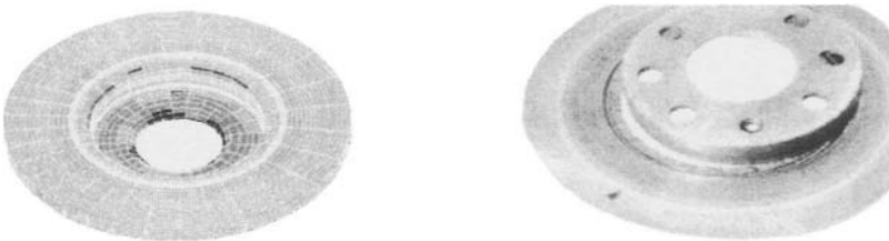
Figure 9 : bowl failure and dissipated energy cartography.
