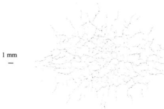
Fig. 6. PWR condition, \Delta T = 200^\circ\text{C} , network observed at the surface, after 150 000 cycles (at the end of the test)
