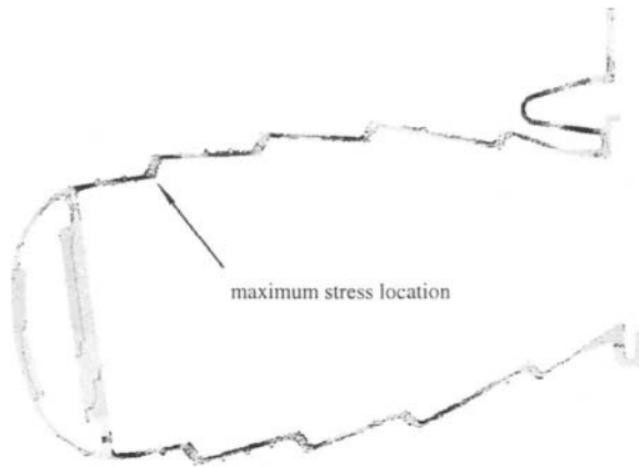
Fig.3: Maximum Stress Location in Combustor from Global Linear-elastic Analysis
