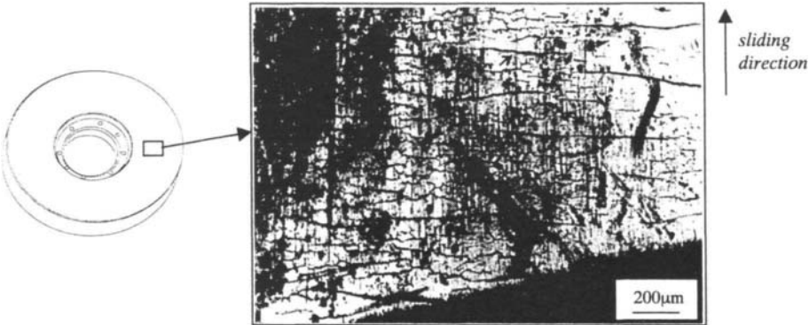
Fig. 2: Friction surface gradually polished
