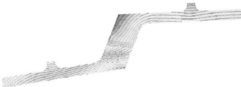
Fig.5: 3D Model of Cooling Ring Segment with Temperature Contours
