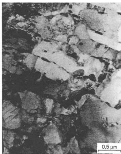
Fig.11. Dislocation microstructure after loading with mean stress 71 MPa and stress amplitude 265 MPa.
