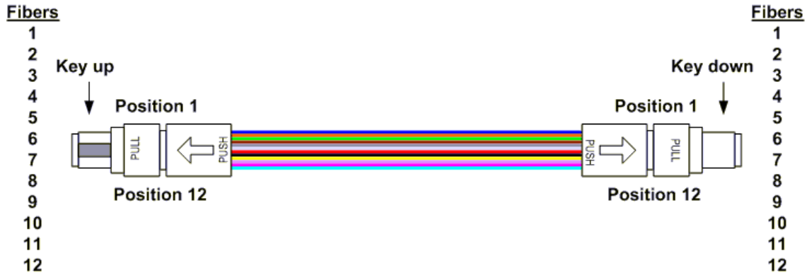
Figure 7 - Type-A array patch cord (key-up to key-down)
