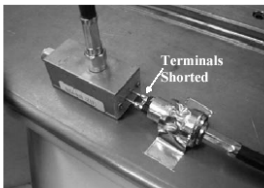
Figure C.10 - Output terminal connection
