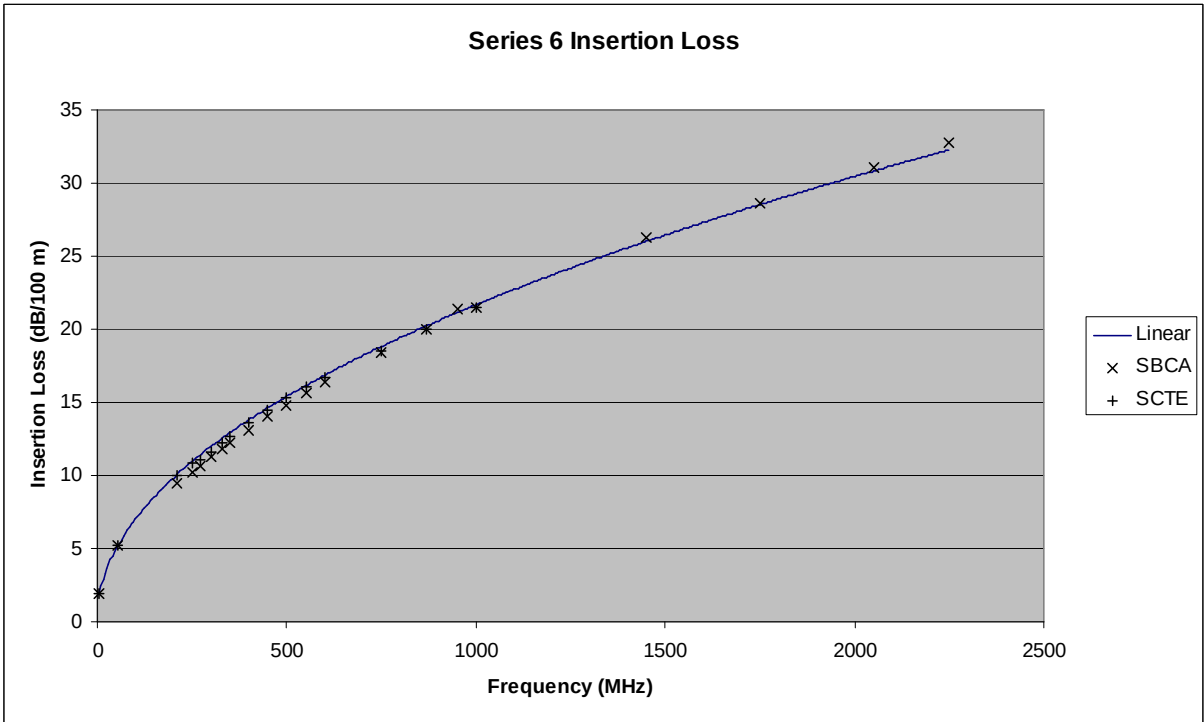
Figure A.1 - Comparison of linear versus discrete insertion loss values, Series 6 cable
