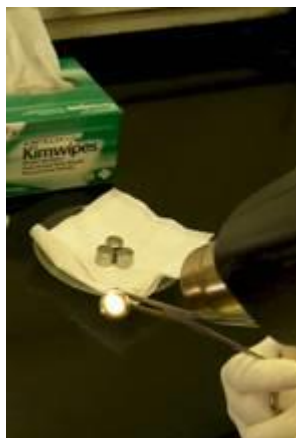
Figure 8: Specimen, held with clean forceps in a gloved hand, being dried by a heat gun. Several dried specimens are temporarily held on an absorbent lint-free laboratory wipe. (10)
