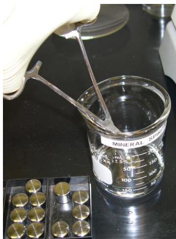
Figure 6: Forceps being used to place prepared steel specimens into the cleaning beaker. (8)
