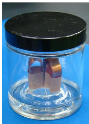
Figure 14: Sealed test jar with three copper panels wrapped with VCI paper samples. (18)
