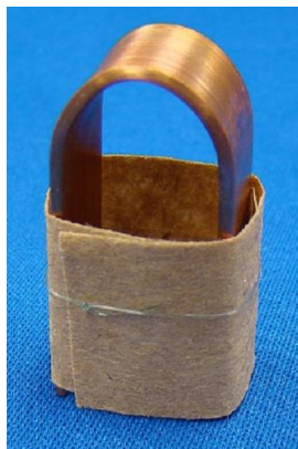
Figure 13: U-shaped copper panel wrapped with VCI paper sample. (17)
