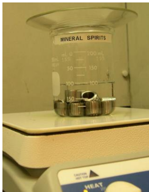
Figure 7: Hot plate with cleaning beaker covered with watch glass to reduce evaporation. (9)
