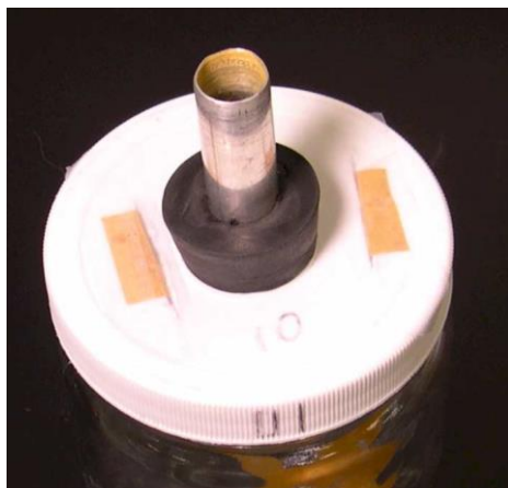
Figure 10: VIA-Ferrous test jar lid (external view) showing VCI material sample strips inserted through slots in lid and held in place with low-acid transparent adhesive tape. (12)
