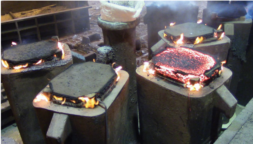
Fig. 7.4 Photograph showing hot top with exothermic boards; note that the board has just burnt through for ingot at bottom right
