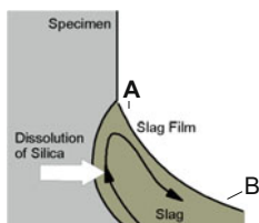
Fig. 11.95 Marangoni convection of slag film in the local corrosion zone of a \text{SiO}_2(\text{s}) –( \text{FeO} – \text{SiO}_2 ) slag system showing typical “slag-line” attack (permission granted, IOM/Taylor & Francis, [250])
