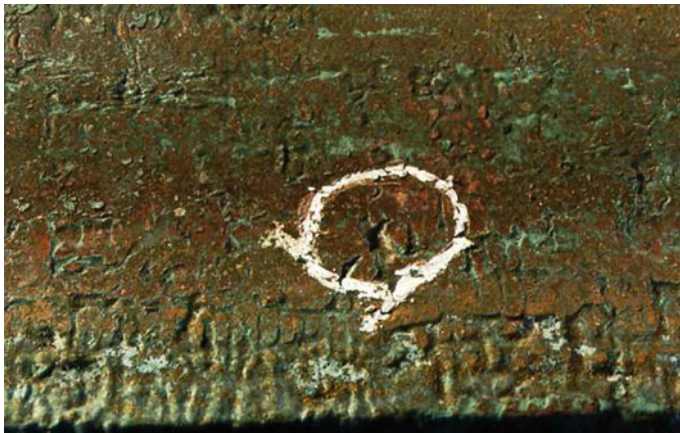
Fig. 6.13 Photograph showing “cavities” in steel surface ( marked ) when using liquid mould slags (permission granted, SWEREA [60])
