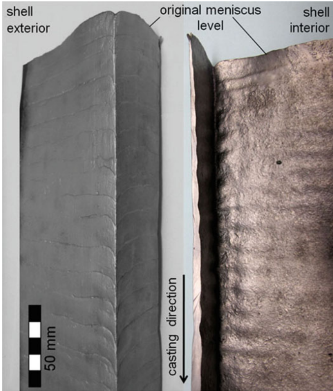
Fig. 11.31 Breakout shell showing internal depressions matching external depressions (permission granted, Taylor & Francis, [103])
