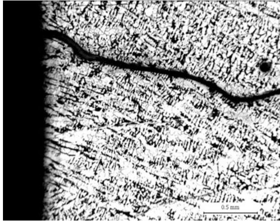
Fig. 11.42 Micrograph showing a transverse crack on the surface of a micro-alloyed, low carbon steel (permission granted, Europ. Comm. Sci. Tech. Publ. [139])
