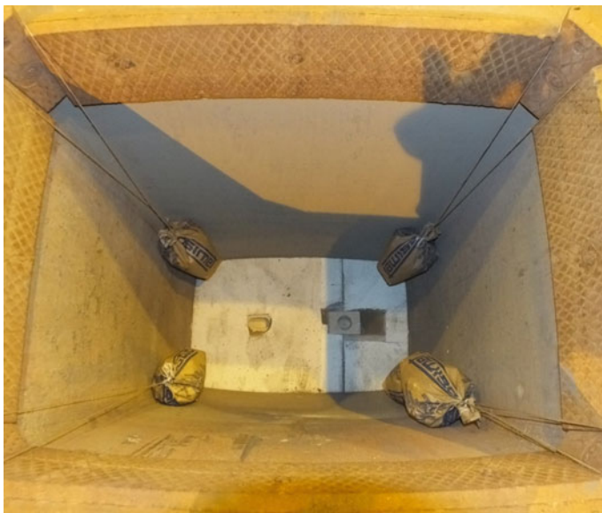
Fig. 7.25 Photograph showing 10 ton ingot mould prepared with mould powders
