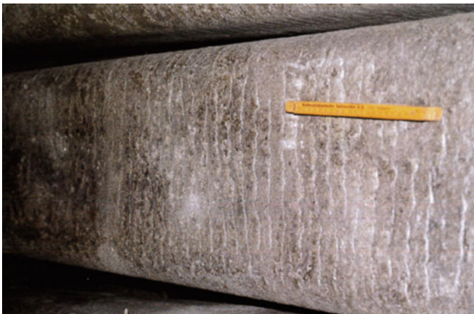
Fig. 7.15 Example of an ingot with strong ripple marks due to mould slag entrainment between mould and ingot [9]
