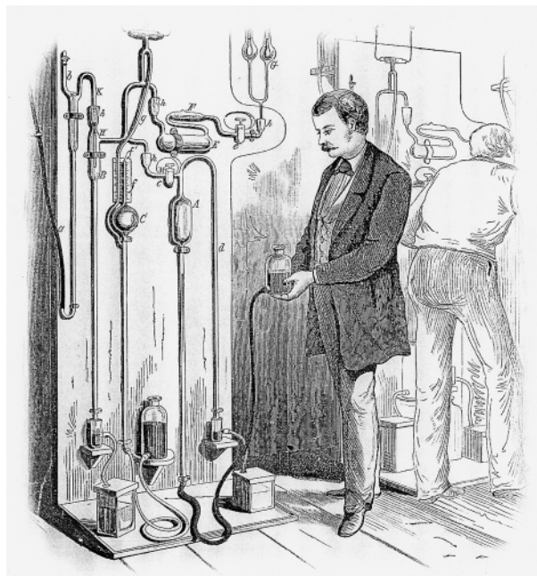
Figure 2. Vacuum pumping, 1880s style. This type of vacuum pumping system was used by T. Edison in the early manufacture of light bulbs.
