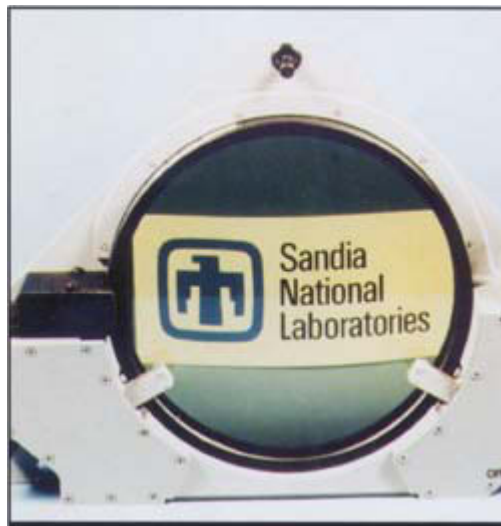
Figure 4-27. Electro-optic lens in the on position, showing the high level of transparency. (Photo courtesy of Sandia National Laboratories, Albuquerque, NM.)
