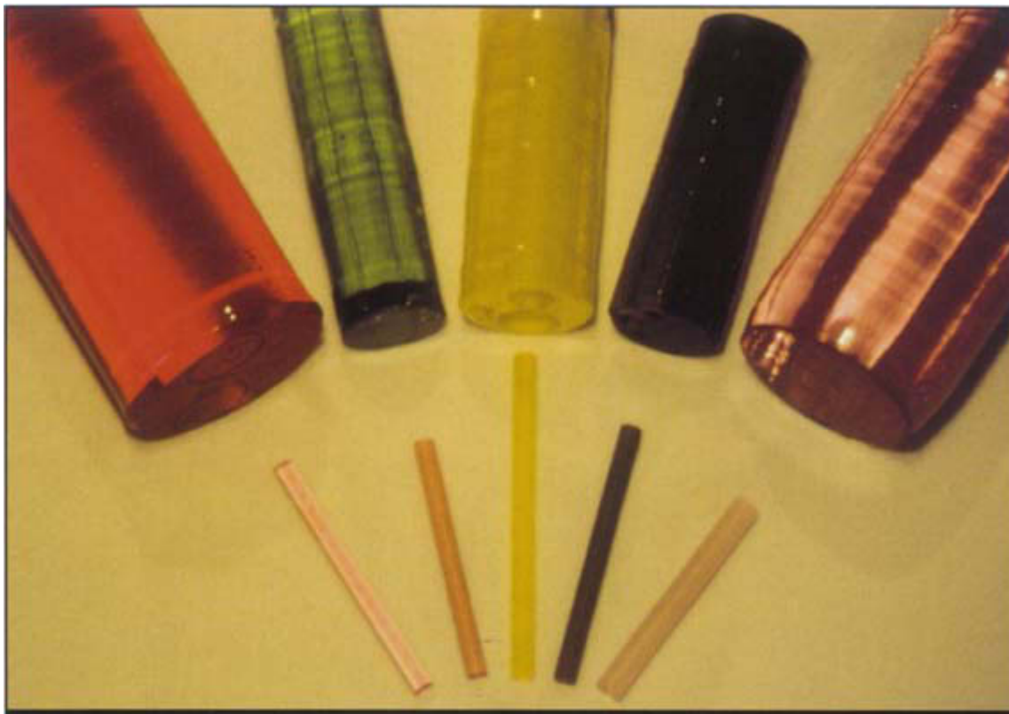
Figure 4-24. Single crystals and laser rods cut from them. (Photo courtesy of Union Carbide Crystal Products, Washougal, WA.)
