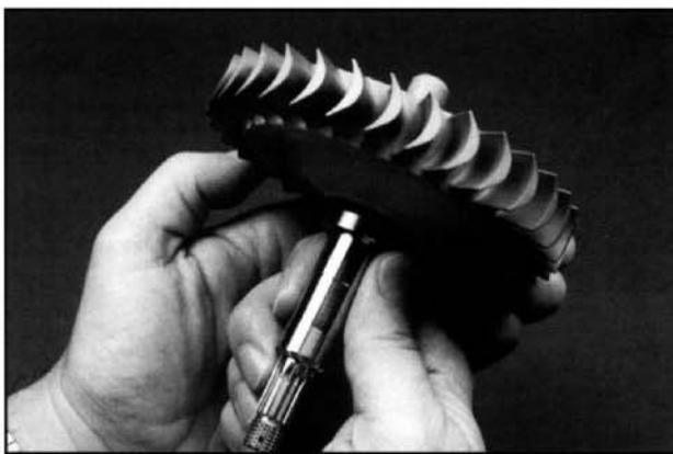
Figure 5-6. Silicon nitride air turbine starter attached to a metal shaft. (Photograph courtesy of AlliedSignal Ceramic Components, Torrance, CA.)
