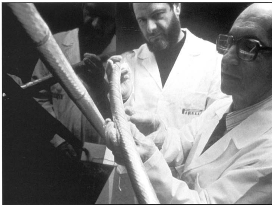
Figure 6-21. Ceramic superconductor wire and experimental electrical transmission line. (Photographs courtesy of American Superconductor Corporation, Westborough, MA, and Pirelli Cavi S.p.A.)
