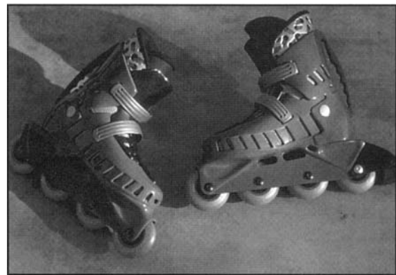
Figure 5-11. Silicon nitride bearings in in-line skates boast record-setting performance and long life. (Photograph courtesy of Saint-Gobain/Norton Advanced Ceramics, East Granby, CT.)
