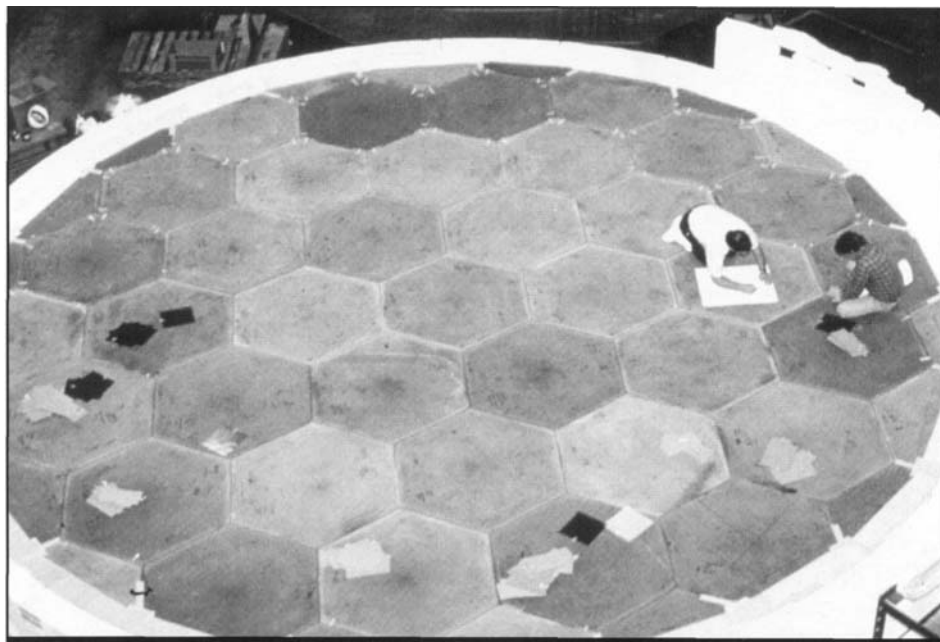
Figure 5-25. Low-expansion glass mirror for the 325 inch diameter Subaru Telescope. (Photo courtesy of Corning, Inc., Corning, NY.)
