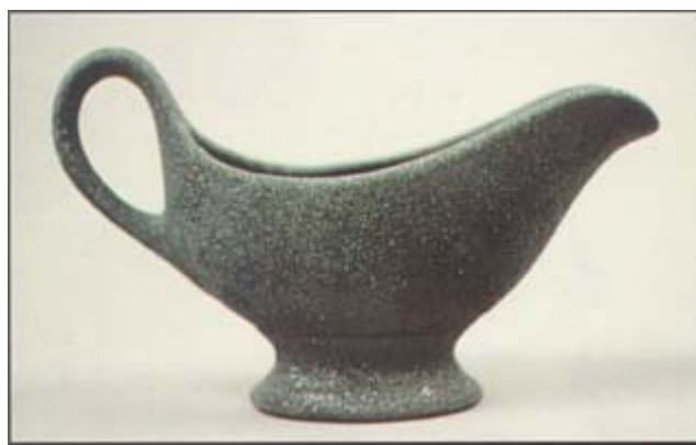
Figure 3-31. Silicon carbide gravy boat. Fabricated by Shenango Refractories, The Pfaltzgraff Company, by slip casting. Measures 7.8 inches long. Originally displayed at a manufacturers' exposition to attract attention and show the shape-forming capabilities of the manufacturer. Donated in 1997 to The International Museum of Art at Alfred and featured in the exhibition Conspicuous Applications of Advanced Ceramics , curated by Dr. William Walker. (Courtesy of the International Museum of Art at Alfred, Alfred, NY.)
