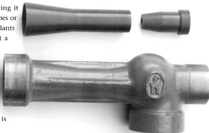
Figure 11-9. Silicon nitride Eductor liners and metal holder for the pneumatic conveying of powdered coal. (Photo courtesy of Ceradyne, Inc., Costa Mesa, CA.)
