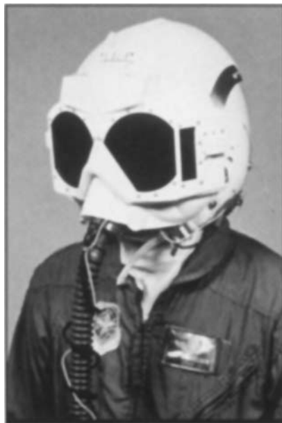
Figure 4-26. Pilot wearing electro-optic goggles in the off position. (Photo courtesy of Sandia National Laboratories, Albuquerque, NM.)
