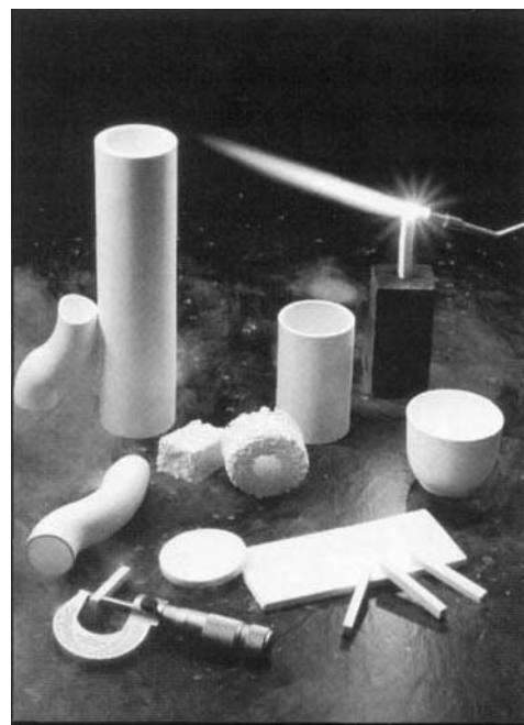
Figure 5-26. Dimensionally stable, low-thermal-expansion NZP ceramic parts. (Photograph courtesy of LoTEC, Inc., Salt Lake City, UT.)
