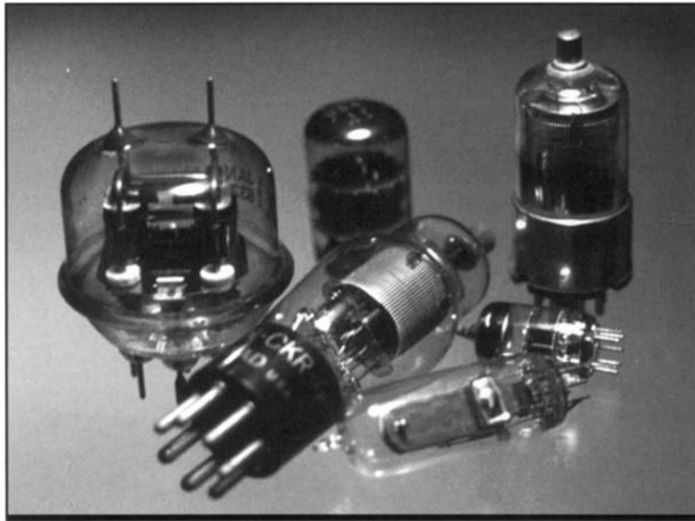
Figure 6-1. Vacuum tubes, showing the metal plates and wires encased in a glass "envelope." Largest tube shown is 4.5 inches high. (Photo by D. Richerson.)
