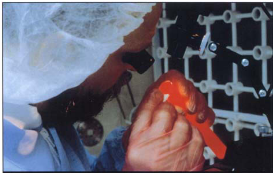
Figure 4-23. Ruby laser rod being inspected. (Photograph courtesy of Union Carbide Crystal Products, Washougal, WA.)
