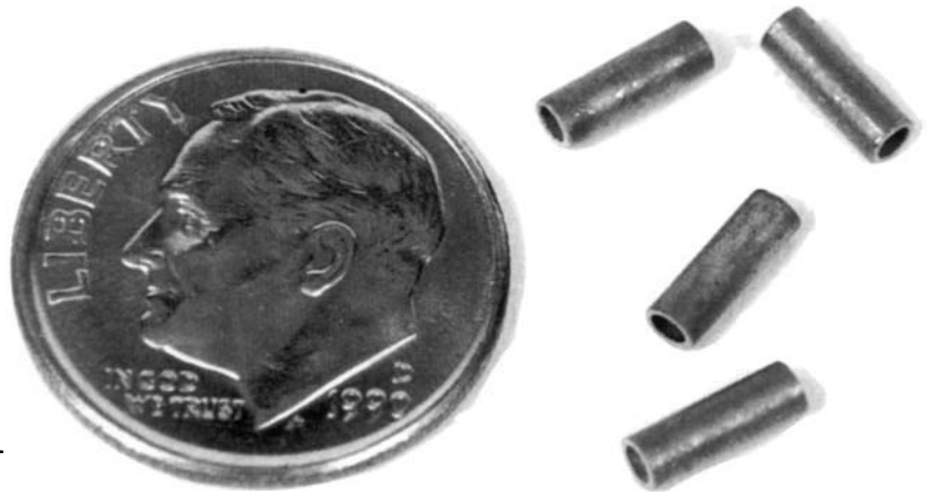
Figure 7-9. Low-cost, miniature sensors for detecting impact or vibration. (Photo courtesy of Edo Corporation Piezoelectric Products, Salt Lake City, UT.)
