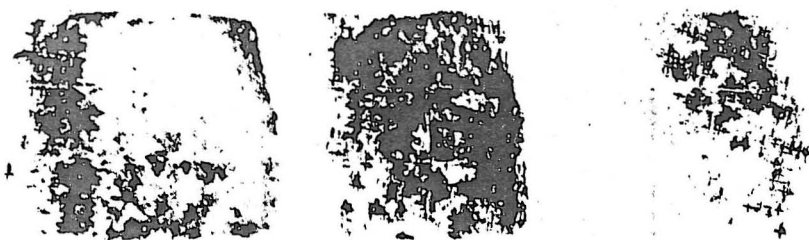
Figure 5.2-8 Monochromatic synchrotron X-ray topographs for the (\bar{1}13) reflection. The middle reference topograph was obtained at the maximum of the diffraction peak, while the one on the left hand side corresponds to a shift of -40^\circ and that on the right hand side to a shift of +20^\circ . The different images are complementary and clearly reveal the formation of groups of dendrites. Courtesy UJF, see also 188 .
