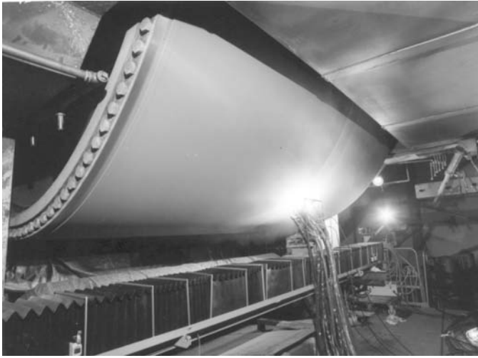
Figure 9.10 A yankee dryer coated, in situ , with an Mo coating, applied by air-plasma spraying. Reproduced by permission of Tocalo Company, Ltd, Kobe Japan
