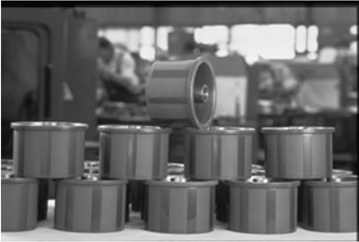
Figure 9.8 Elements for guiding textile fibres coated with ceramics. Reproduced by permission of Terolabservices, Villeneuve-Le-Roi, France
