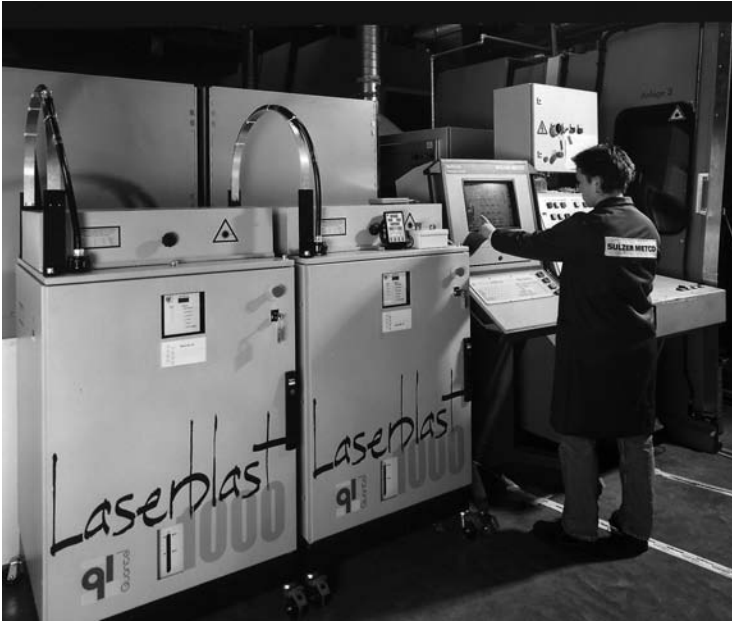
Figure 2.9 A Laserblast TM installation for laser cleaning and activation of substrates. Reproduced by permission of Quantel, Les Ulis, France
