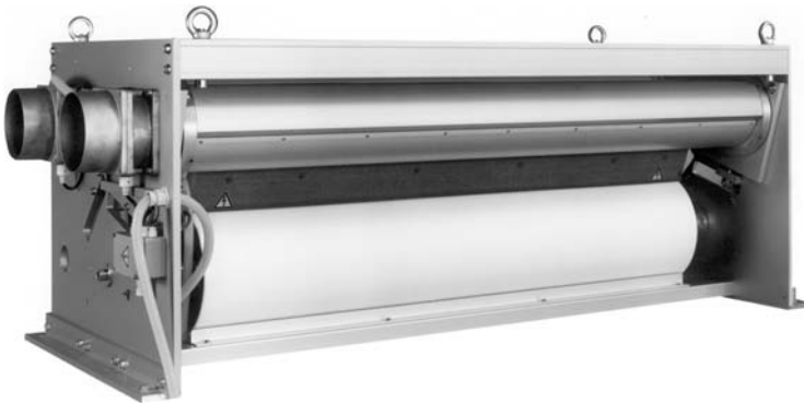
Figure 9.12 A corona ‘treater’ with a roll coated with electrically conducting alumina. Reproduced by permission of Softal Electronic GmbH, Hamburg, Germany
