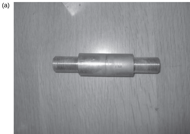
Figure 7.9 Views of (a) two specimens 'glued' together before testing, (b) installed in the loading fixture of a tension machine and (c) the two specimens after rupture
