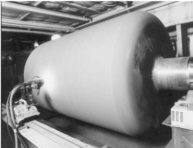
Figure 9.7 A continuous annealing line roll during deposition of \text{Cr}_3\text{C}_2 cermets using atmospheric-plasma spraying (external diameter of about 800 mm and a length of about 4500 mm). Reproduced by permission of Tocalo Company, Ltd, Kobe Japan
