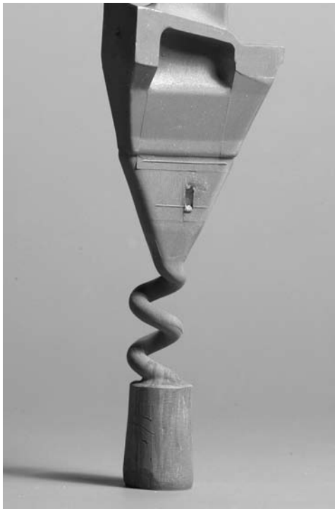
Fig. 3.6. Details of the starter block and pig-tail grain selector from the Trent 800 high-pressure turbine blade casting.
