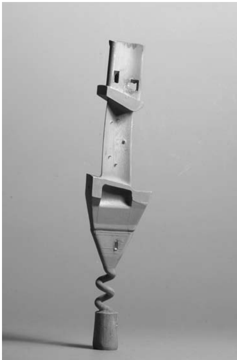
Fig. 3.5. Rolls-Royce Trent 800 high-pressure turbine blade casting, after removal of the investment shell.
