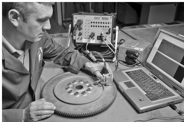
Figure 10.4 Eddy current testing of a geared wheel component (© TWI).
