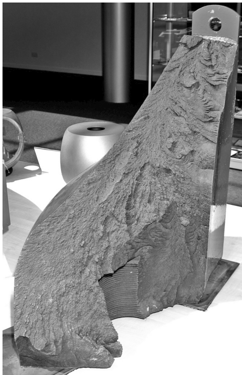
Figure 8.6 A piece salvaged from the John Thompson pressure vessel failure in 1965, now on display at TWI, Cambridge. The thick section forging shows a classic brittle fracture appearance with river lines pointing towards an initiation point at or beyond the location that the lifting lug has been attached (© TWI).
