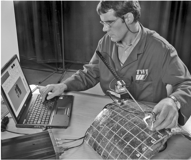
Figure 10.6 Ultrasonic probe being used to scan a component to quantify the extent of wall thinning owing to internal corrosion (© TWI).
