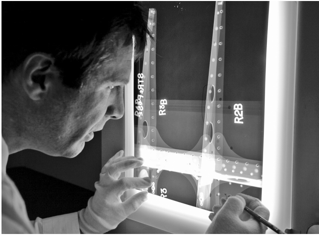
Figure 10.5 Radiograph image being examined over a light box. This image is of a riveted aircraft component (© TWI).
