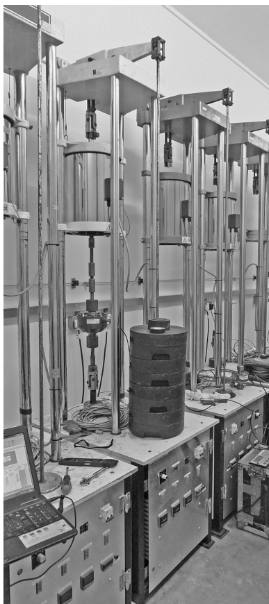
Figure 9.11 Creep testing rig, under a deadweight load during calibration. During creep testing the heating component cylinder is brought down to surround the test specimen seen in the middle of the picture (© TWI).
