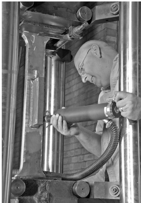
Figure 13.7 Ultrasonic peening around the weld toes of a fillet welded attachment to a fatigue test specimen (© TWI).
