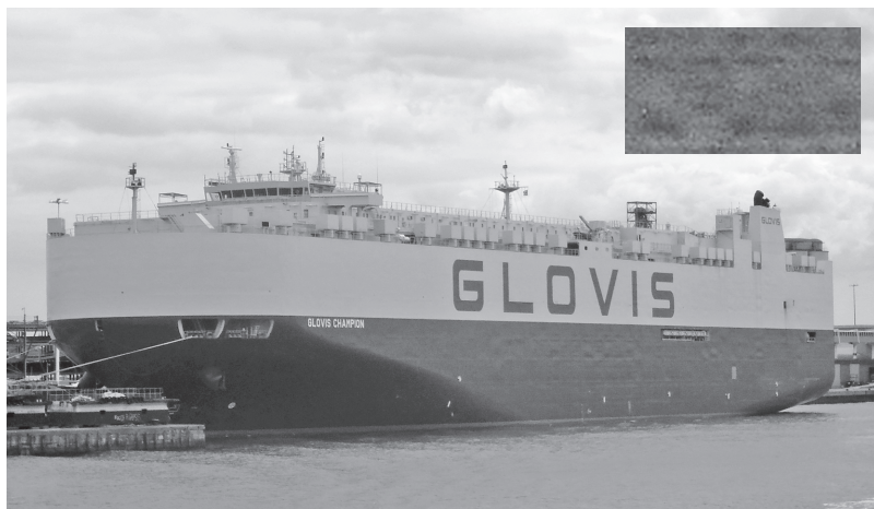
Figure 3.8 The Glovis Champion vehicle carrier (built in 2013) showing ripples and distortion of the lower hull panels (see magnified portion of hull underneath the ‘OV’ of ‘GLOVIS’) caused by welding (© TWI).
