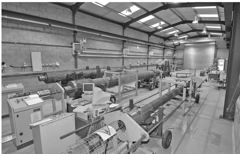
Figure 9.10 Resonance fatigue testing of pipeline girth welds. Full-scale test specimens are cyclically loaded using an eccentric load at one end until resonant frequency is achieved, such that a large number of stress cycles can be imposed on the pipe in a short time (© TWI).
