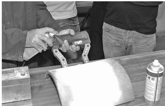
Figure 10.3 Magnetic particle inspection (MPI): a suspension of magnetic particles sprayed onto a weld, to which a magnetic field is being applied from a permanent magnet. The weld has previously been painted white in order to show up any defects (© TWI).
