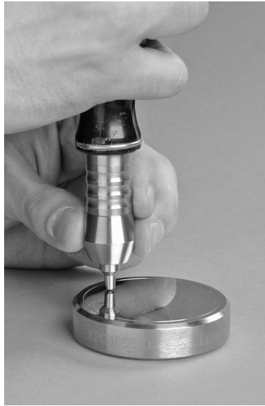
Figure 9.16 Microdur portable surface hardness testing equipment supplied by GE Inspection Technologies (© TWI).
