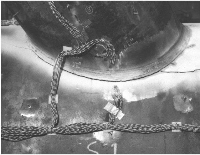
Figure 7.15 Fatigue test on a tubular welded connection, showing strain gauges attached to record the stresses at different locations on the structure (© TWI).
