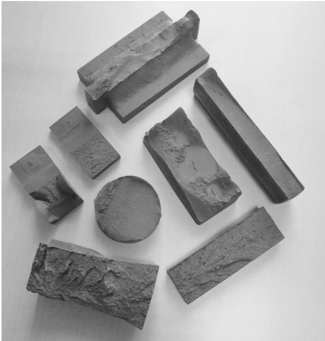
Figure 8.13 TWI's plastic fracture replica set, used during training courses to recognise ductile, brittle and fatigue failure modes (© TWI).
