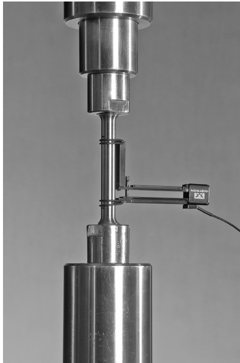
Figure 9.2 Round tensile test specimen fitted with an extensometer across the gauge during a tensile test (© TWI).
