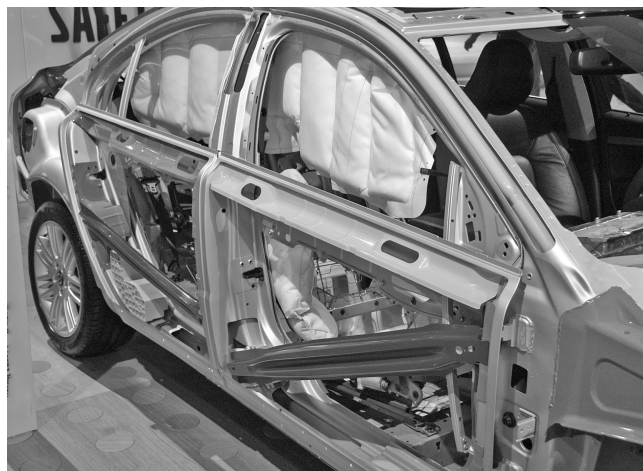
Figure 2.3 Side impact protection bars in a car frame, (darker diagonal bars) (© TWI).
