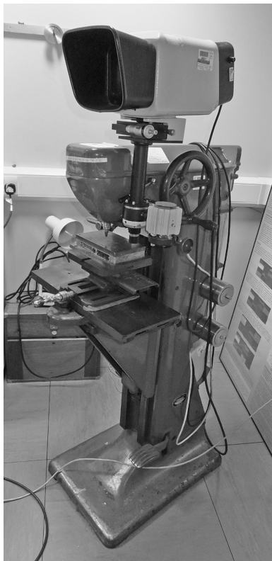
Figure 9.14 Vickers hardness testing machine (© TWI).
