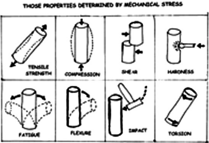
Fig. 6.2 Mechanical properties determined by mechanical stress, Everything is Material . Cleveland Ohio: ASM Materials Education Foundation, page 108
