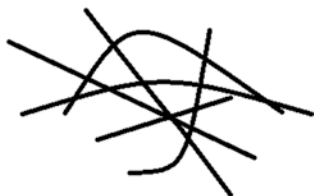
Fig. 1.3 Representation of uncured molecules as a result of the influence of a shear force, demonstrating the effects of a force being applied to a non-Newtonian fluid. Everything is Materials, page 21 of solids, ASM Educational Foundation
