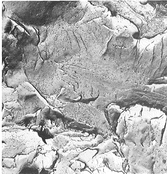
Figure 18 – Quasi-cleavage in Zircaloy-2
