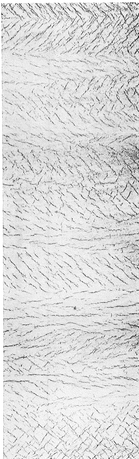
Figure 3 (a) – Hydride Orientation Observed on a Transverse Section Through the Wall of a Quenched and Aged Zr-2.5 Wt% Nb Pressure Tube, Viewed in Optical Microscopy.
