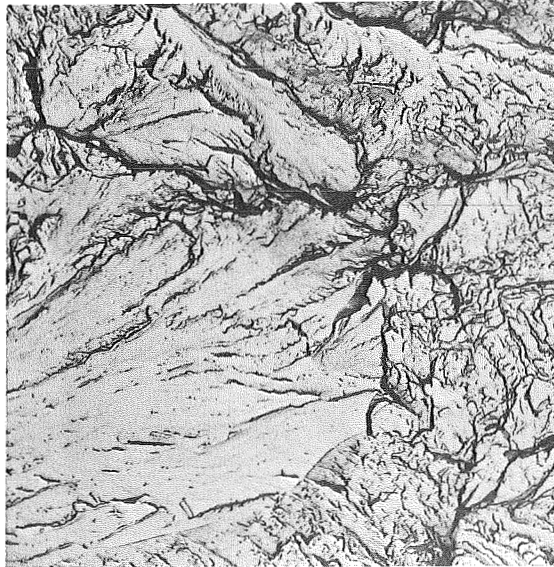
Figure 14 – Feather cleavage at start of fatigue crack (3000 X)
