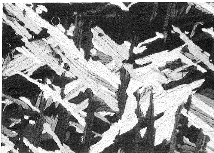
Figure 4 – Widmanstätten structure in Zircaloy-2 slowly cooled from the \beta phase (500X)
