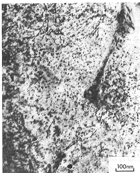
(a) Zircaloy-2 (1.0 - 1.5% Sn in solid solution)
