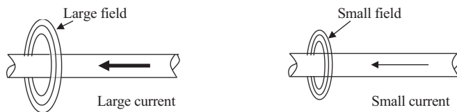
FIGURE 1.5 The strength of the magnetic field around a wire carrying a current depends on the amount of current.
