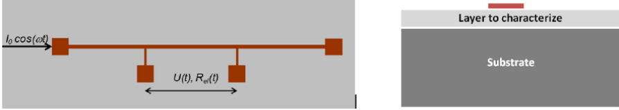
Figure 4.77. Diagram of a typical device for the 3\omega method
