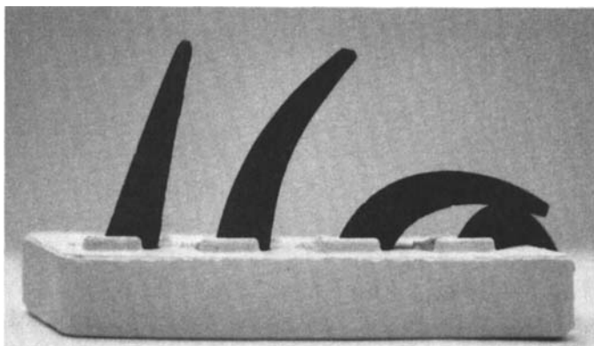
Figure 1.1: Orton pyrometric cones [4].
