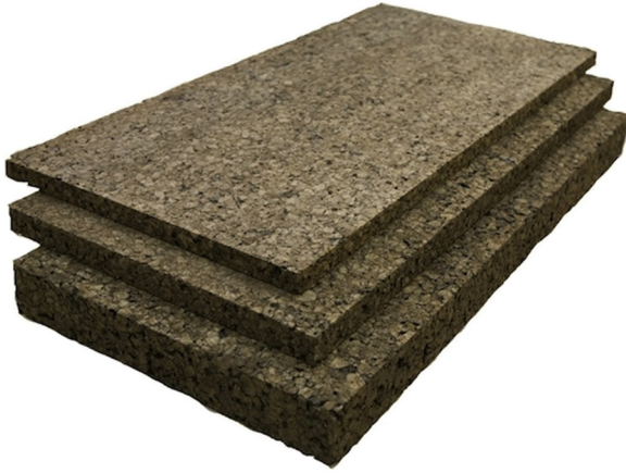
Figure 3.6 Corkboard and cork pipe thermal insulation. (Source: Modern Enviro, Co. )
