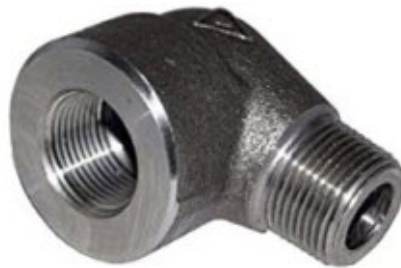
Male/female elbow Dimensions: ASME B16.11 Sizes: 1/8" to 2"
