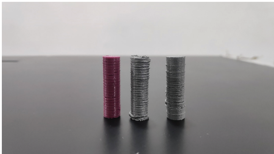
FIGURE 3.1 Pin-on-disk samples before wear testing.
