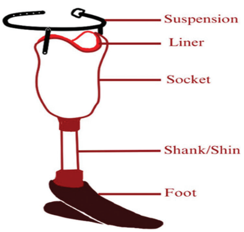
FIGURE 12.4 Customized transtibial prosthetic limb (Fardan et al. 2023).
