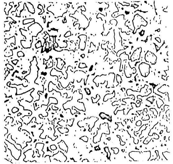
CHILL CAST AND PERMANENT MOLD 100 X MAGNIFICATION
