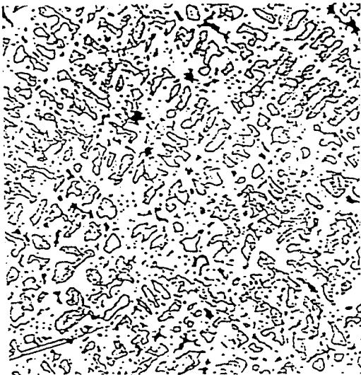
CENTRIFUGAL CASTING 100 X MAGNIFICATION
