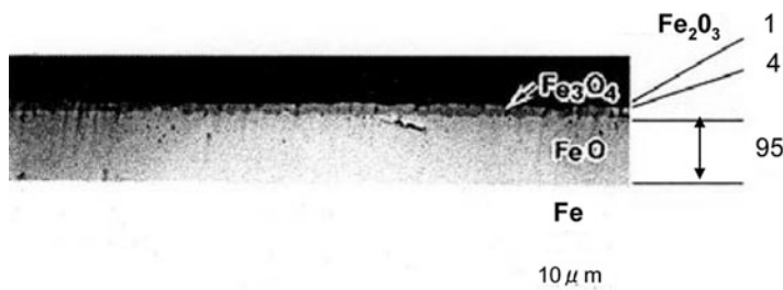
Fig. 5.51 Photographs of cross section of scale on sheet surface of low carbon steel
