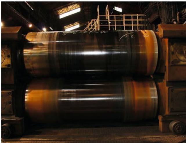
Fig. 5.66 Black scale layer on work roll in tandem mill
