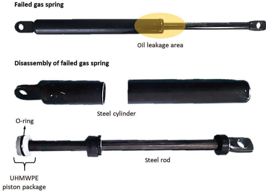
FIGURE 2.9 Detailed views of the failed gas spring.
