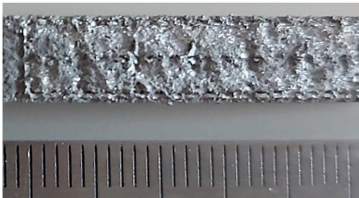
FIGURE 5.3 SLM manufactured Ti6Al4V surface after trimming support structures.
