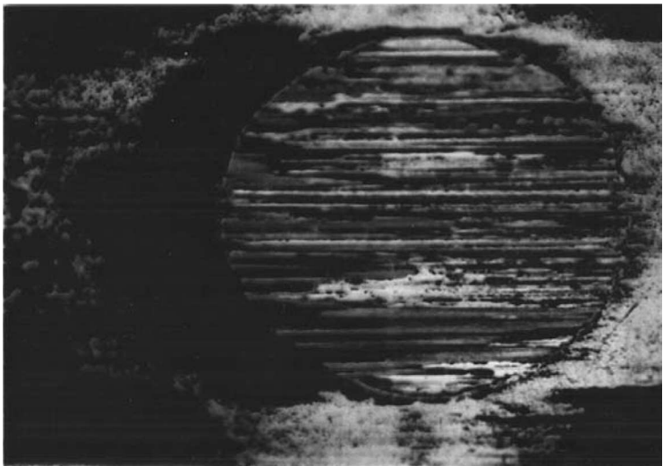
Figure 9.18 Carbon transfer layer and debris particles on and around wear scar formed on steel ball slid against DLC film
