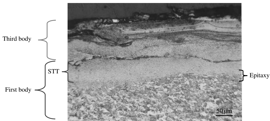
Figure 12.6 STT and third body obtained in a wheel–rail contact: longitudinal cross-section of the wheel [reproduced by permission of Dr. Yves BERTHIER]
