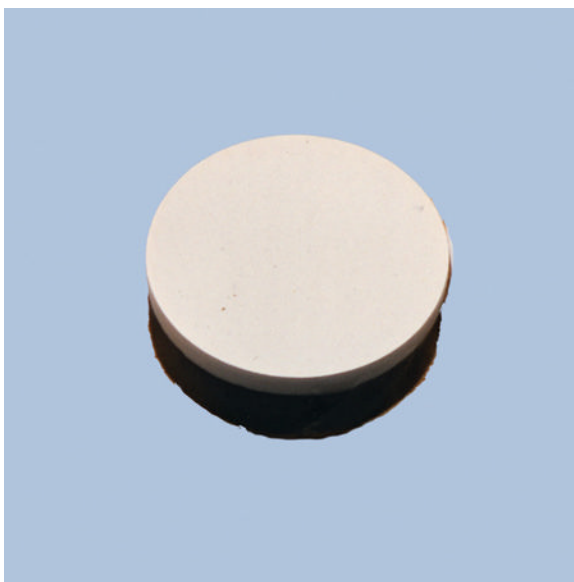
Figure 14.8. Optical photograph of \text{HfN}_{0.95} after 3 min arcjet exposure at 2000^{\circ}\text{C} showing an adherent oxide scale [78].
