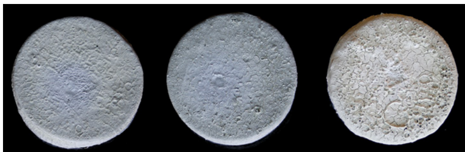
Figure 7.5. The 30 mm diameter×20 mm thick, Cf-HfB 2 composites after 60 s oxyacetylene torch testing at >2500°C showing negligible surface erosion.
