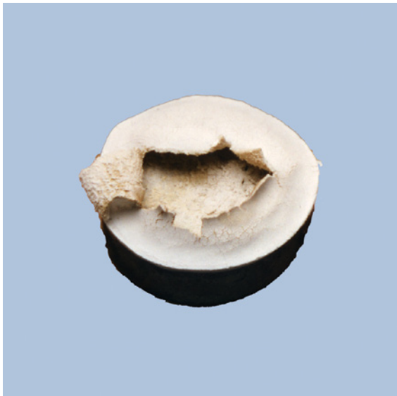
Figure 14.10. Posttest micrograph of \text{HfN}_{0.75} showing oxide scale disruption (Wuchina E, Opeka M. Unpublished data).
