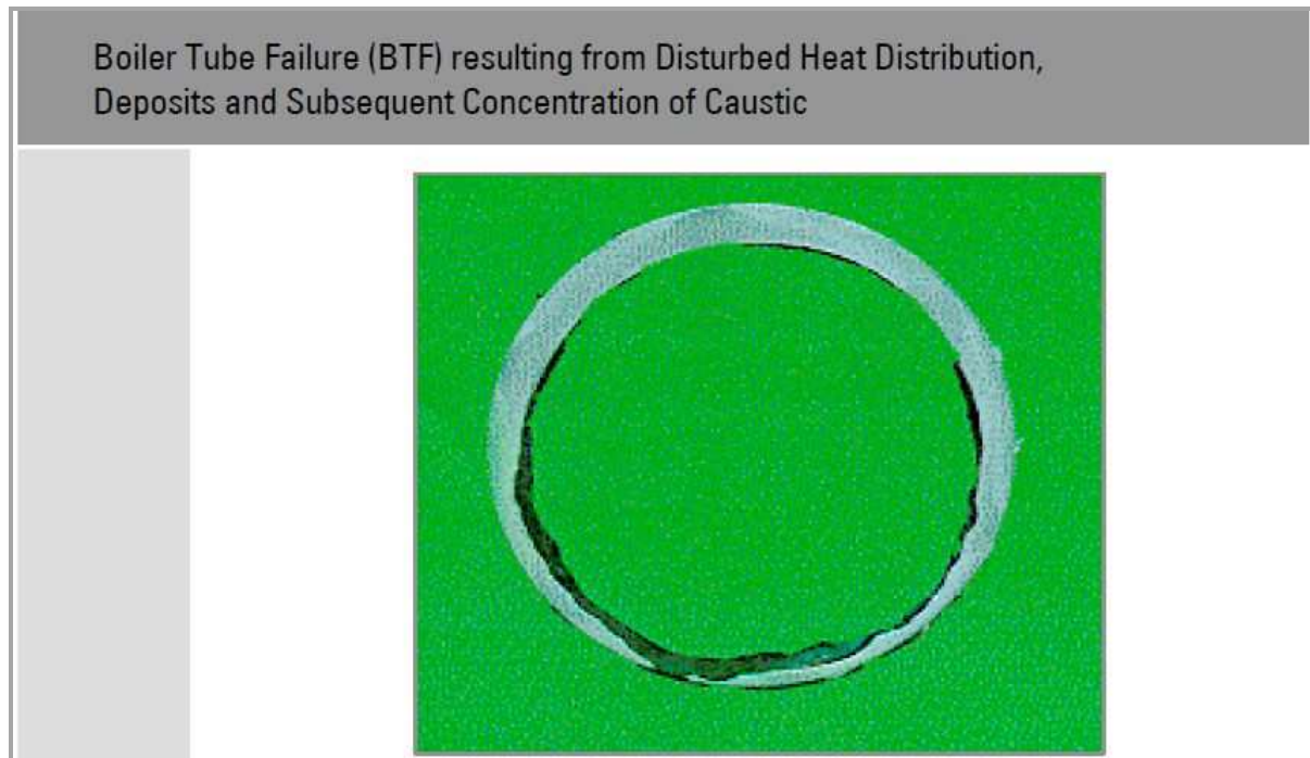
Figure 42: Example – shrinkage of material thickness.
