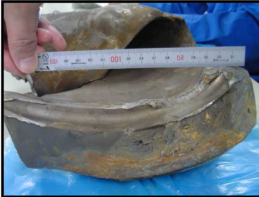
Figure 40: Example – fatigue break.
