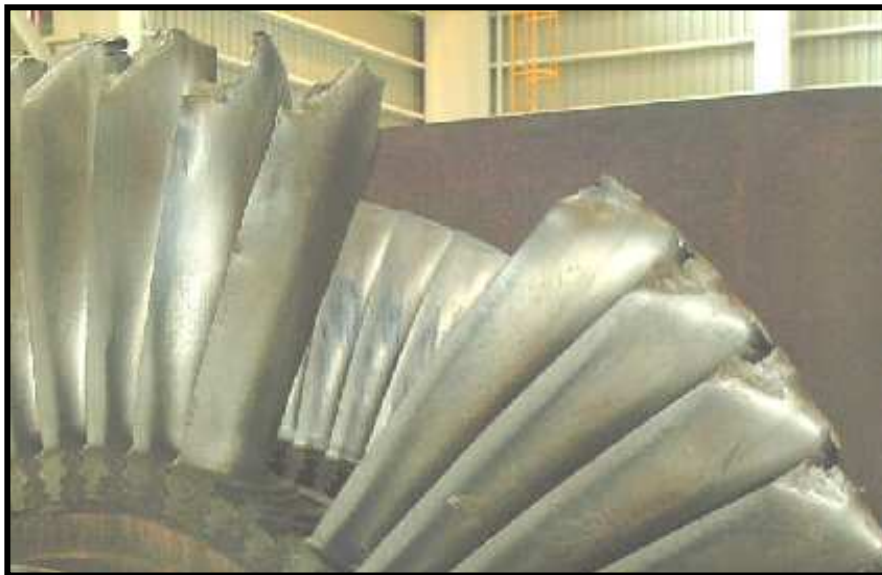
Figure 41: Example – notch effect.
