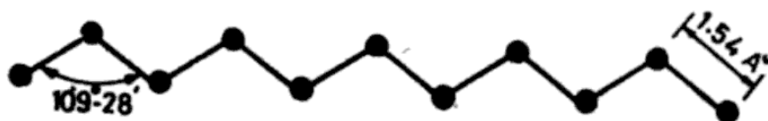
Fig. 3.12 Fully extended form of a polymer chain made of C—C backbone comprising ten C—C bonds.
