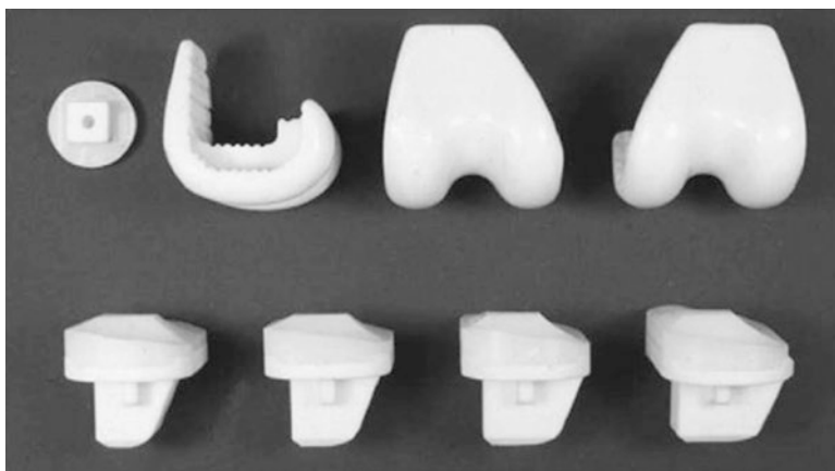
Fig. 4.3 Implants made from alumina ( \text{Al}_2\text{O}_3 ) [4]
