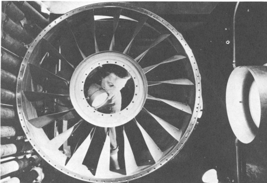
Figure 8.3 Inspection of inlet assembly of aircraft gas turbine using ultra-violet light after application of fluorescent penetrant. (Courtesy of Magnaflux Ltd.)
