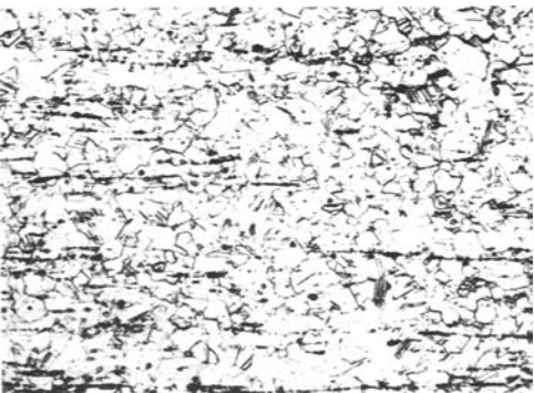
Fig. 13 Microstructure of material adjacent to the weld and at the fracture surface shown in Fig. 10(b). 122 \times
