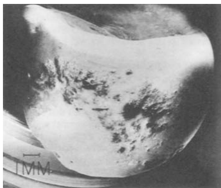
Fig. 18 Copper-aluminum alloy restoration after intraoral usage showing the severity of plaque buildup that can occur. Source: Ref 68
