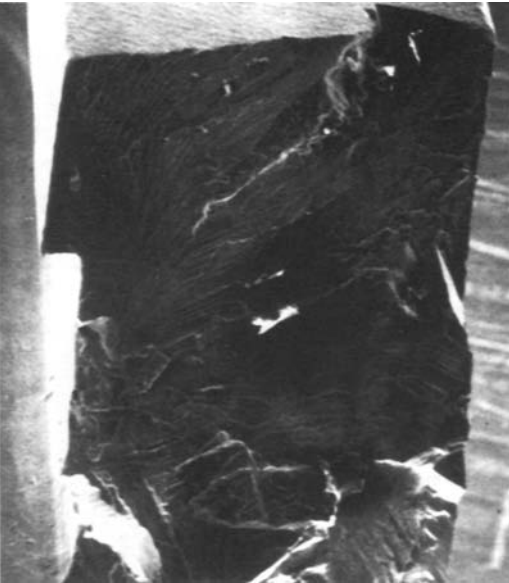
Fig. 69 Low-magnification micrograph of crack-initiation region at base of capture lip in a titanium-alloy tibial component
