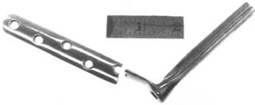
Fig. 7 As-received Jewett nail implant
