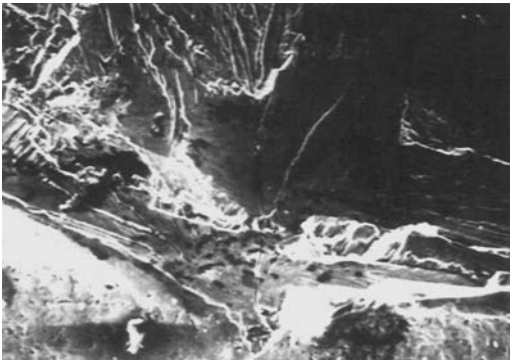
Fig. 71 Higher-magnification view of Fig. 70. Note appearance of large prior- \beta grain in initiation region.
