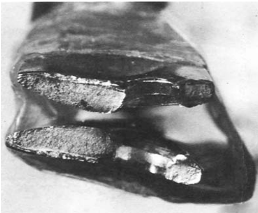
Fig. 8 Mating fracture surfaces. 14.24 \times . Failure initiated on the outside (convex) surface and progressed across the plate thickness by low-cycle fatigue. \sim 15\times
