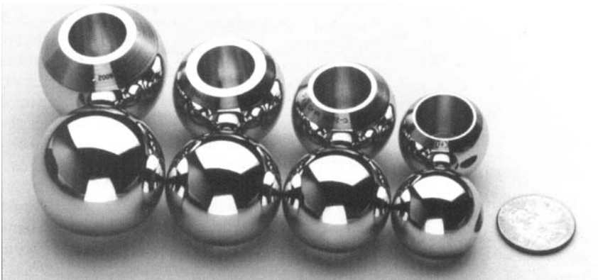
Fig. 10 Femoral bearing caps made from hot isostatically pressed Co-Cr-Mo alloy (ASTM F 799). Source: Carpenter Technology Corporation
