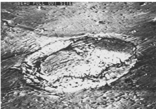
Fig. 72 Micrograph of surface of titanium-alloy tibial tray where a sintered bead has fractured off. Note incomplete fusing of the bead to the tray.
