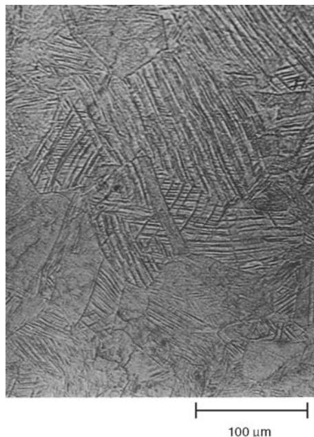
Fig. 1 Microstructure of cold-worked AISI type 316L stainless steel. Etchant: 20 mL HCl, 10 mL HNO 3 , and 3 g FeCl 3 for 2 to 5 s
