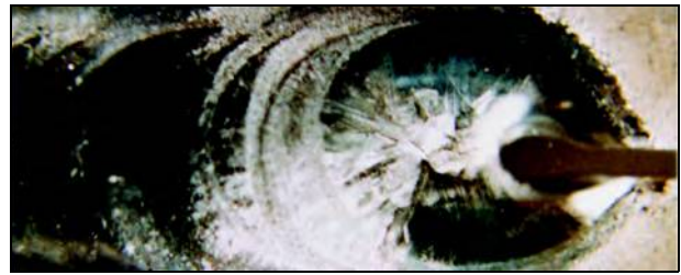
Figure 9.6—Closeup of Crater Cracks in Aluminum Weld
