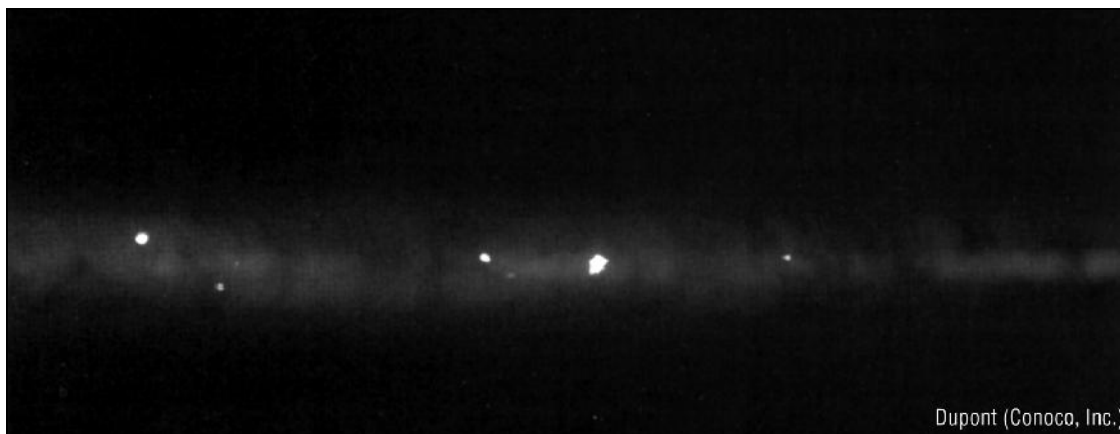
Figure 9.22—Radiographic Image of Tungsten Inclusions
