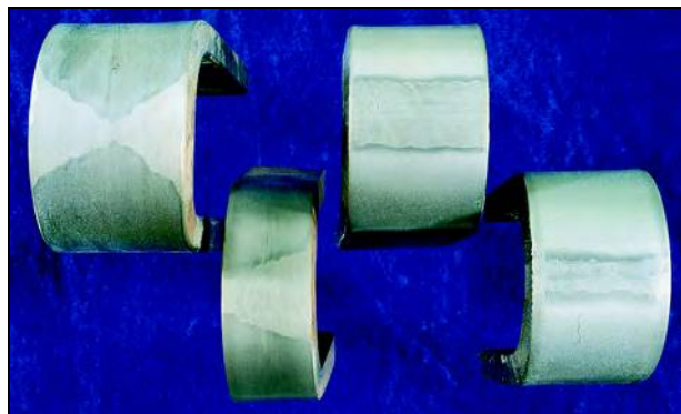
Figure 6.24—Typical Transverse Weld Bend Specimens
