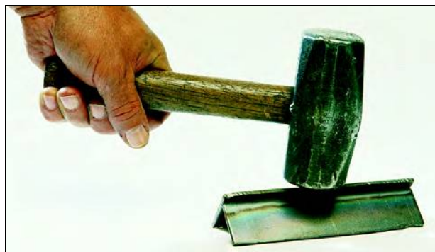
Figure 6.31—Method of Rupturing Fillet Break Specimen
