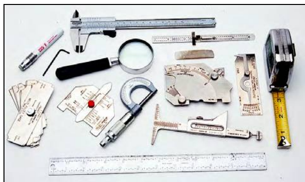
Figure 10.2—Visual Inspection Tools
