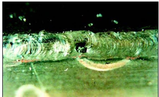
Figure 9.19—Surface Slag Inclusion
