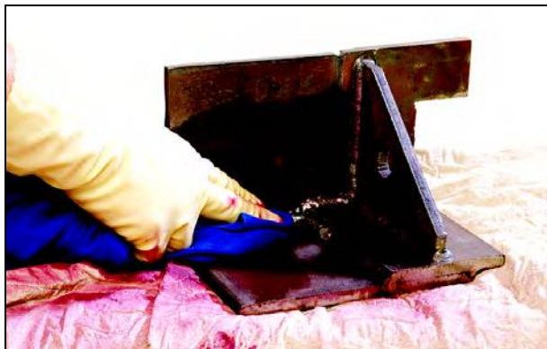
Figure 10.17—Excess Penetrant Removed
