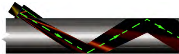
Figure 10.34—Angle Beam Propagation
