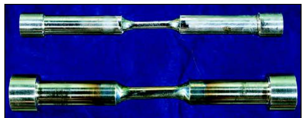
Figure 6.2—Tensile Specimen with Reduced Section
