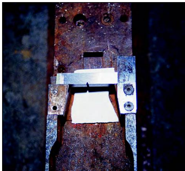
Figure 6.17—Placement of Charpy Specimen in Anvil
