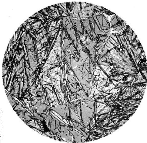
Figure 8.10—Quenched Martensite—Showing Acicular Structure (500X)
