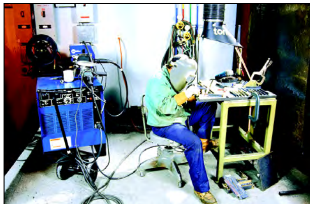
Figure 2.3—Designated Welding Area
