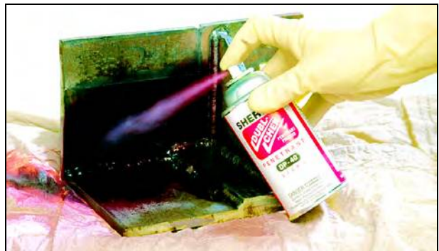
Figure 10.16—Penetrant on Test Surface and In Crack
