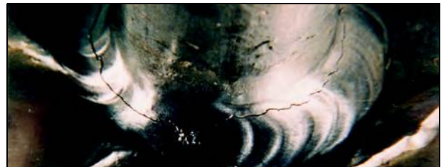
Figure 9.7—Propagation of Crater Crack in Aluminum Weld
