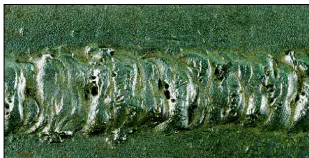
Figure 9.25—Isolated Surface Porosity
