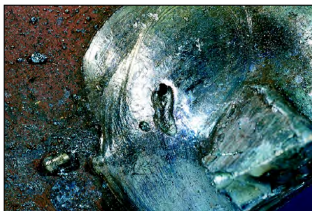
Figure 9.26—Elongated Surface Porosity
