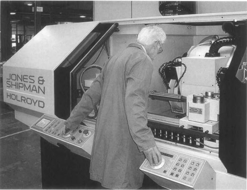
Figure 11.6 A Jones & Shipman—Holroyd Suprema Easy CNC cylindrical grinding machine during set-up (with permission).
