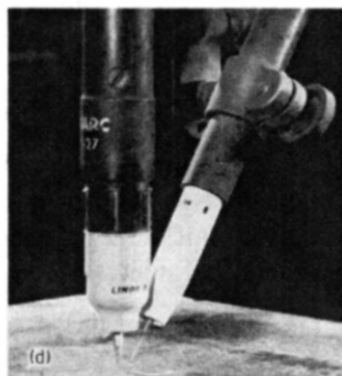
33 Commercially available hot wire TIG equipment: a) Manual system with single power source and integral wire feed; b) Manual torch; c) Mechanised system with separate power sources for arc and wire; d) Mechanised head with separate torch and wire feed nozzle.
