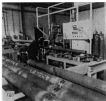
36 Hot wire TIG welding of cast reformer catalyst tubes: a) General view of welding equipment; b) Joint preparation (courtesy of APV Paramount Ltd).
