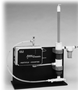
Figure 4 Typical drinking water particle counting system
