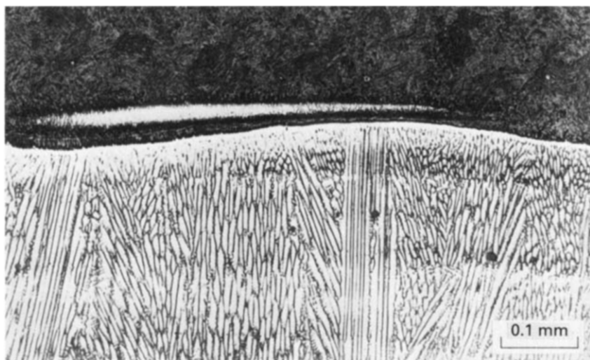
1.7 Tongue of unmixed parent metal in a non-matching weld pool.
