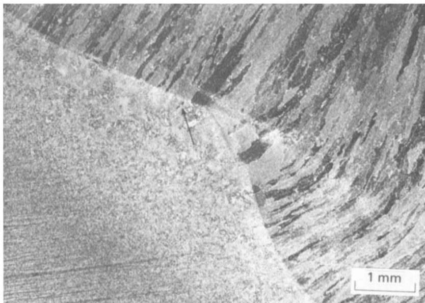
3.25 Liquation crack (arrowed) in bay area of submerged arc weld bead.
