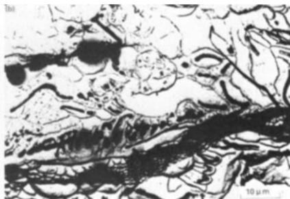
3.41 Crack surfaces in TEM showing: (a) Nb 4 C 3 on solidification crack surface; (b) α-MnS in weld metal ahead of crack tip.
