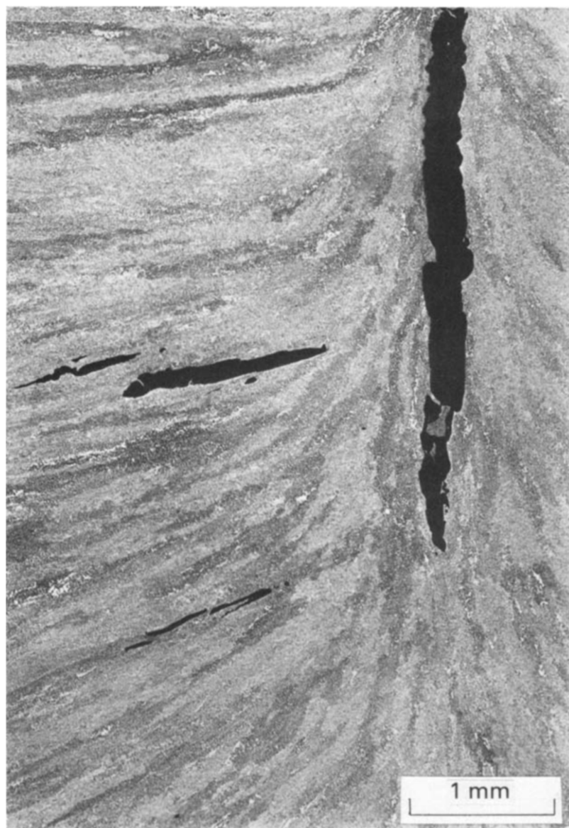
3.13 Detail of cracks of Fig. 3.9 showing relatively blunt crack tips.
