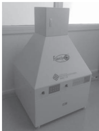
6.30 Image analysis system for the measurement of dimensional stability.
