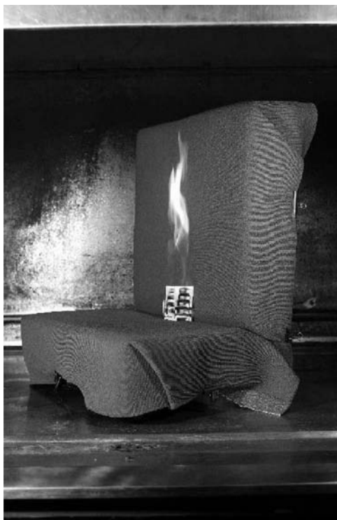
12.15 Composite specimen with wooden crib as ignition source.
