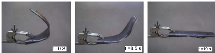
Figure 9.6 Recovery of ESS-SMP Composite skin [60]. ESS, elastic steel slice.
