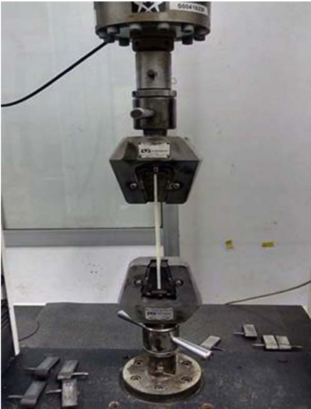
Figure 7.10 Specimen is clamped by the machine.
