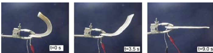
Figure 9.7 Recovery of shape memory alloy (SMA) wire–shape memory polymer (SMP) composite skin [60].
