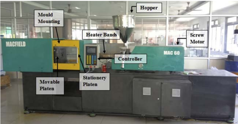
Figure 11.4 Injection moulding machine available at Centre for Composite Materials, Kalasalingam Academy of Research and Education.
