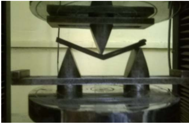
Figure 8.8 Three-point bending test for Mode II [12].
