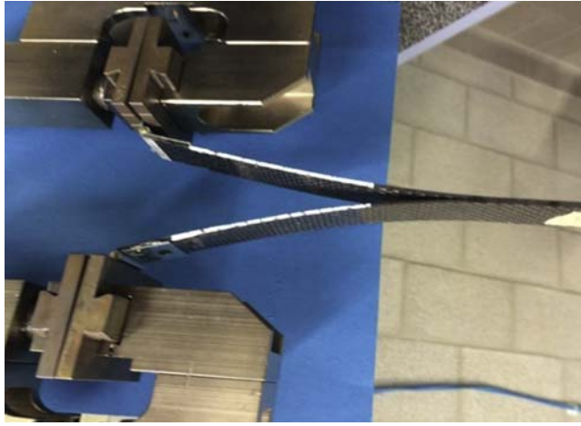
Figure 8.6 Photograph of Mode I test [12].
