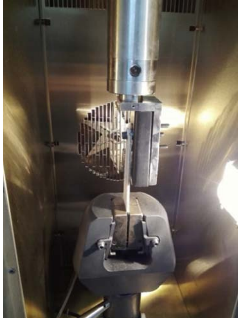
Figure 4.5 Setup of specimen inside the heat chamber.
