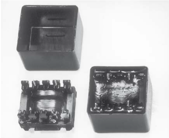
Figure 14.13. Transformer before and after potting
