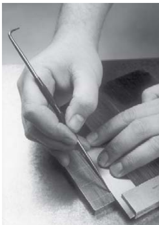
Figure 3.14. Scribing line square to datum
