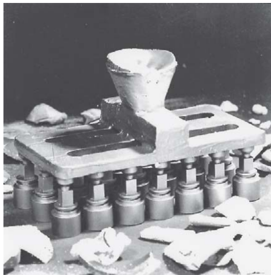
Figure 17.6. Refractory removed from cast metal
