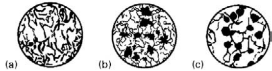
Figure 13.7. Cast irons (a) grey (b) malleable (c) spheroidal-graphite
