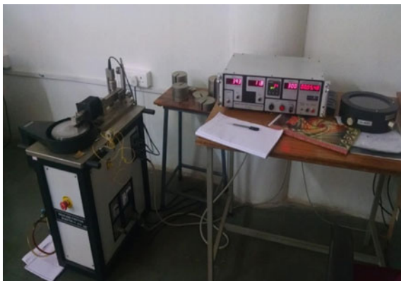
Fig. 4 Disk type wear testing machine
