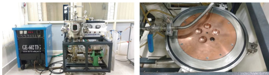
Fig. 1 Experimental setup of vacuum arc melting and copper die
