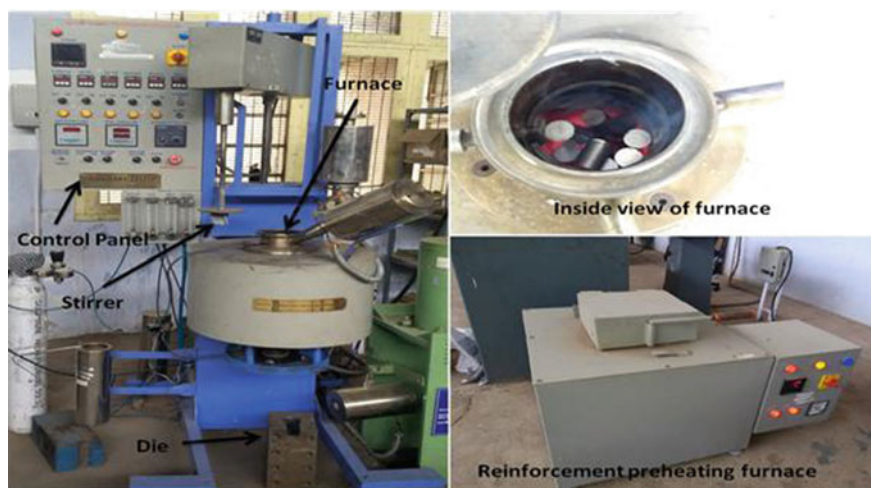
Fig. 1 Stir casting setup
