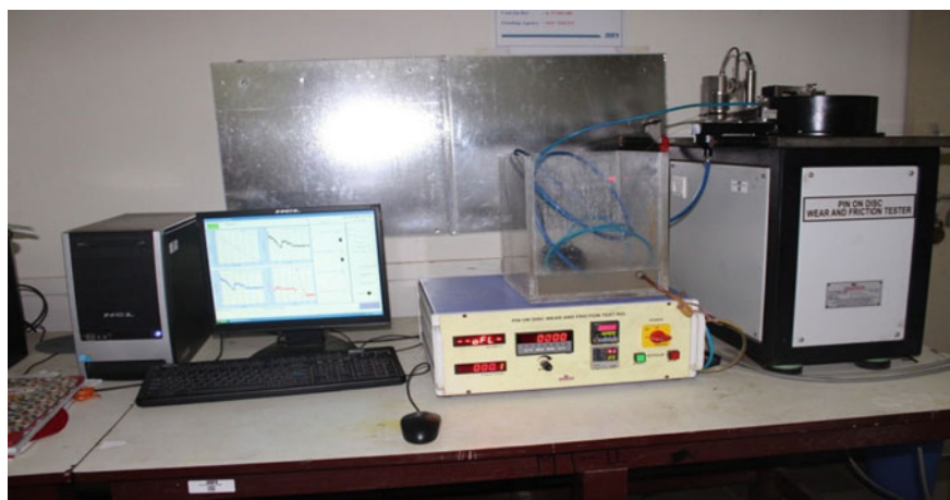
Fig. 2 Computer-assisted pin-on-disc wear tester
