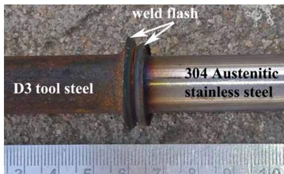
Fig. 2 The photograph of the friction welded joint showing the weld flash at interface
