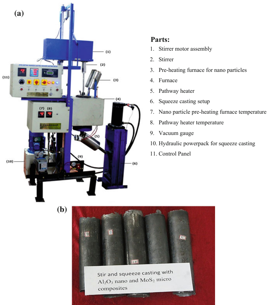
Fig. 1 a Stir and squeeze casting machine, b hybrid composites blanks
