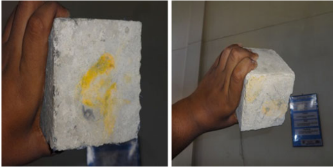
Fig. 7 Concrete cubes before and after cyclic heating @ 50 °C for 7 days
