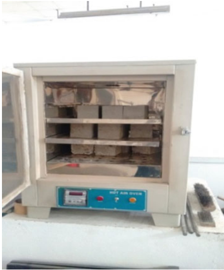
Fig. 5 Concrete cubes in hot air oven for cyclic heating @ 50 °C for 7 days
