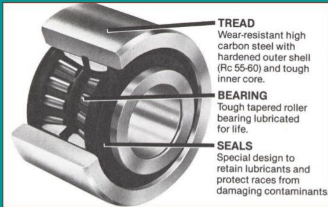
Load runners (idler-rollers)
