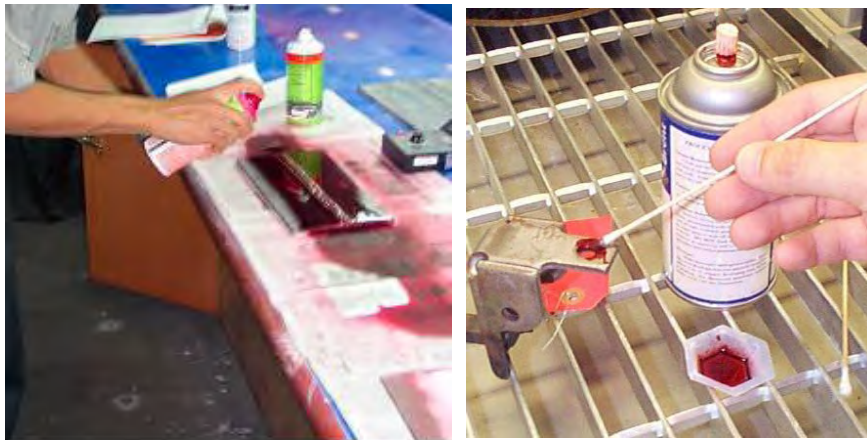
Methods of applying the red dye during dye penetrant inspection.
