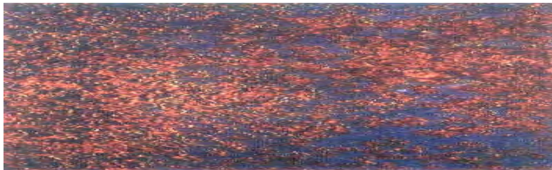
Rust Grade B: Steel surface, which has begun to rust, and from which mill scale has begun to flake.
