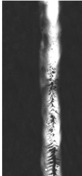
X-ray of a welded seam showing porosity.
