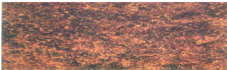
Rust Grade D: Steel surface on which mill scale has rusted away. General pitting visible under normal vision.
