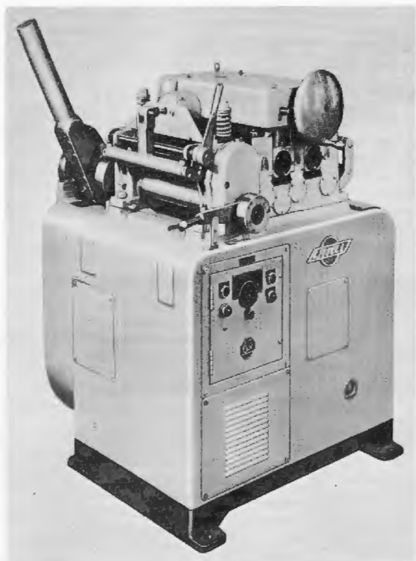
Fig. 2-41. Heavy-duty feeding and straightening machine. F. J. Littell Machine Co.
