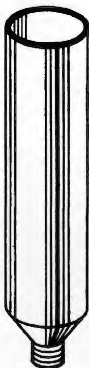
Fig. 1-44. Drawn shell that has been extruded.
