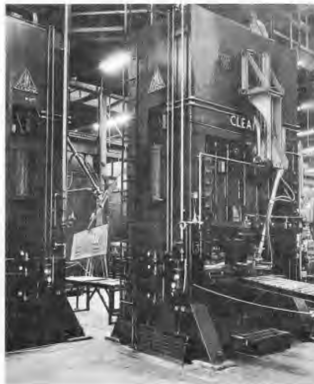
Fig. 2-44. "Iron Hand" unloaders removing parts from presses.
