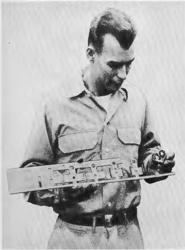
Fig. 1-27. Examining a scrap strip.
