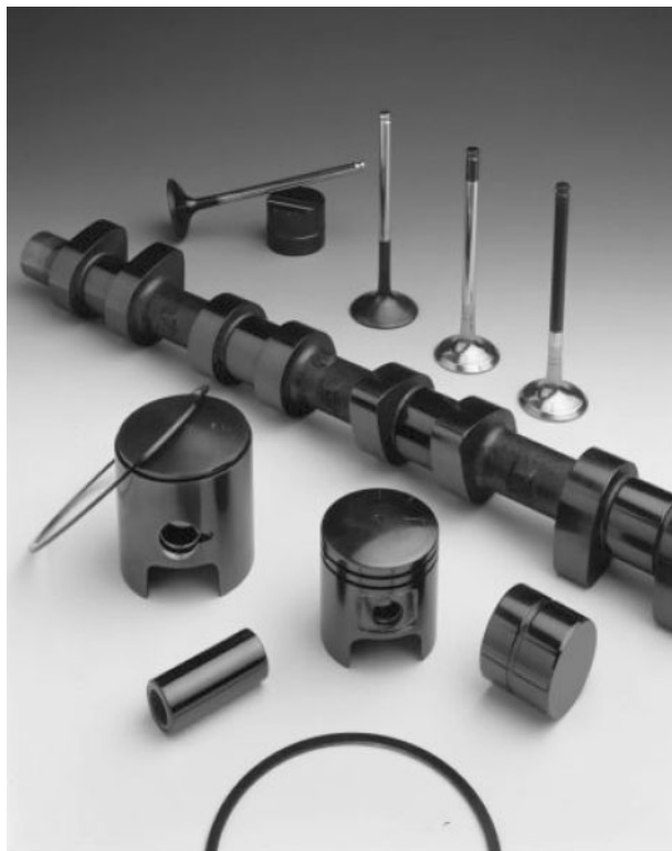
24 Selection of automotive engine components that have been coated successfully with DLC (reproduced with kind permission of Kronos Racing)
