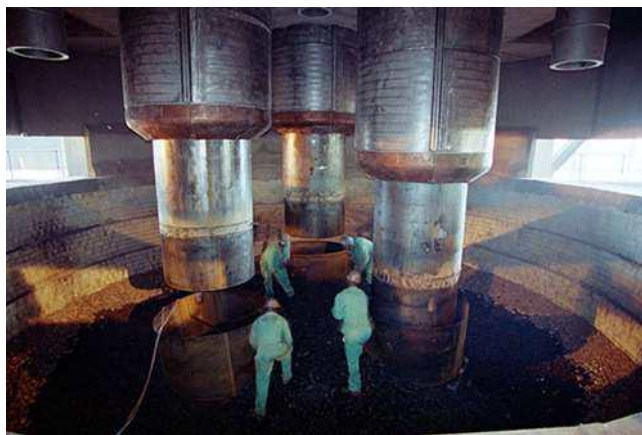
FIGURE 4.3 Circular AC ferrochrome furnace showing the lining and electrodes. (By permission of Tenova Pyromet, a division of Tenova Minerals [Pty] Ltd.)
