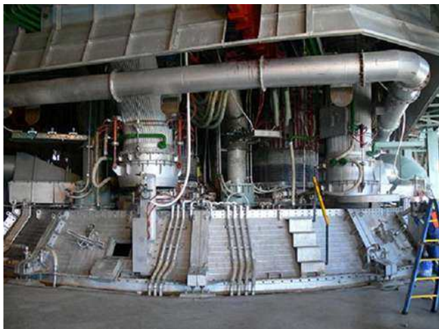
FIGURE 4.5 Closed roof on a FeCr furnace. (By permission of Tenova Pyromet, a division of Tenova Minerals [Pty] Ltd.)
