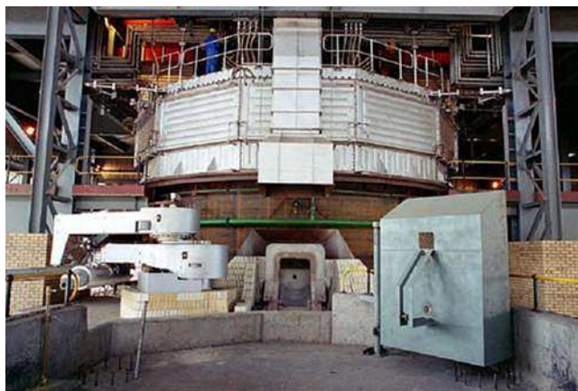
FIGURE 4.7 A ferrochrome furnace viewed from the tapping bay. (By permission of Tenova Pyromet , a division of Tenova Minerals [Pty] Ltd. )
