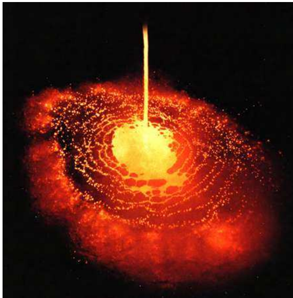
FIGURE 9.12 View of Granshot granulation process. (Source: Uvân Hagfors Teknologi [UHT]. )
