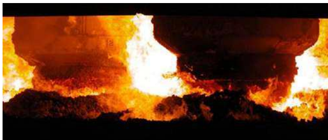
FIGURE 4.2 The furnace in operation showing the electrodes passing into the furnace charge. (By permission of Tenova Pyromet, a division of Tenova Minerals [Pty] Ltd.)
