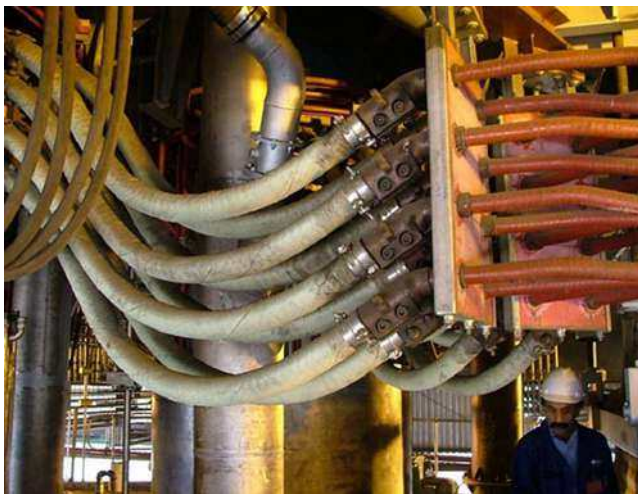
FIGURE 4.14 Flexible water-cooled copper conductors at the electrodes. (By permission of Tenova Pyromet, a division of Tenova Minerals [Pty] Ltd.)
