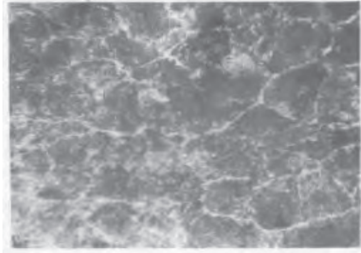
(c) Hypereutectoid steel (pearlite with network of cementite), \times 500 .
