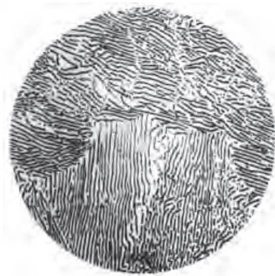
Figure 4.2 Microstructure showing lamellar nature of pearlite ( \times 1200 ).
