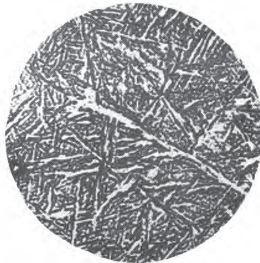
Figure 5.6 Microstructure showing coarse accicular martensite ( \times 300 ).
