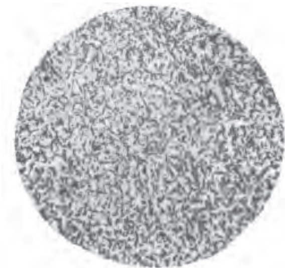
Figure 4.23 Microstructure of lower bainite ( \times 500 ).
