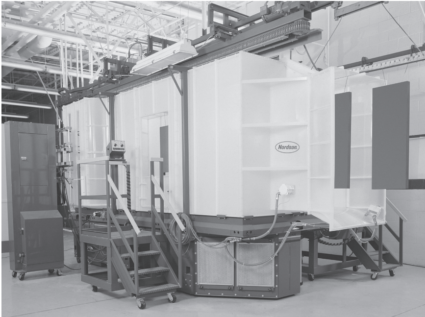
Figure 11-3. Conveyorized booth with manual/automatic guns. (Courtesy Nordson Corp.)
