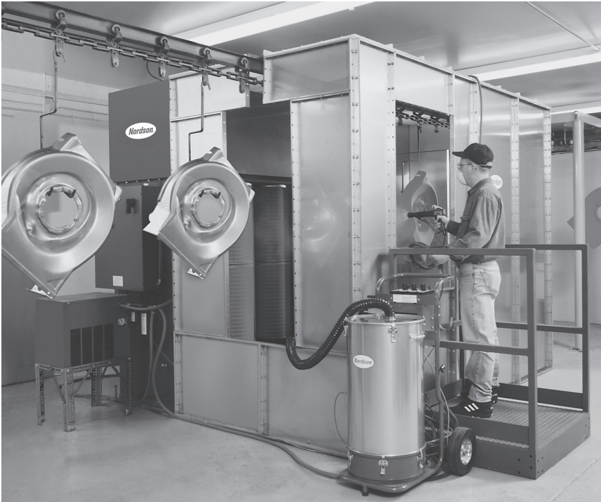
Figure 11-4. Booth for manual-spray operation. (Courtesy Nordson Corp.)
