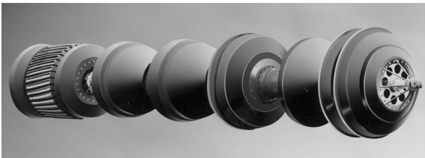
Fig. 17–12. Crack detection pig (Pipetronix, Stutensee, Germany)
