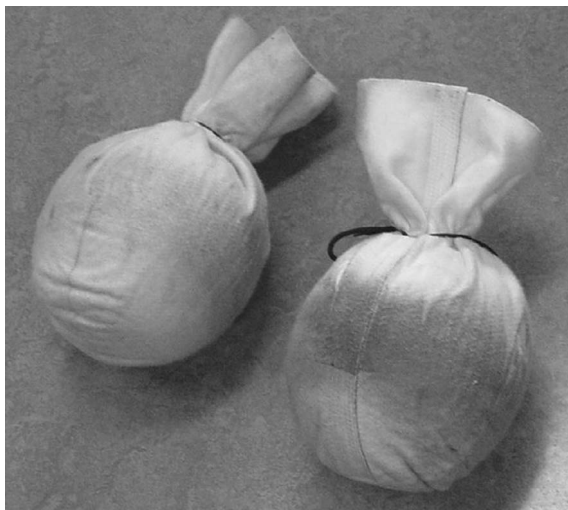
Fig. 18–10. Soft pigs (Coperion- Waeschle, Weingarten, Germany) before (left) and after travel
