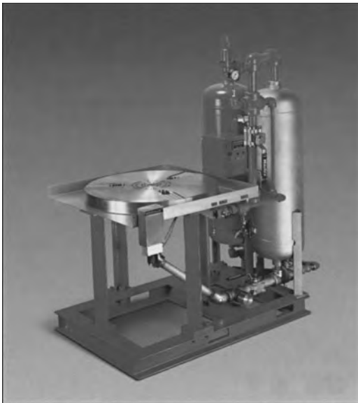
Figure 20.1 A package test stand. (Courtesy: Farris Engineering.)
