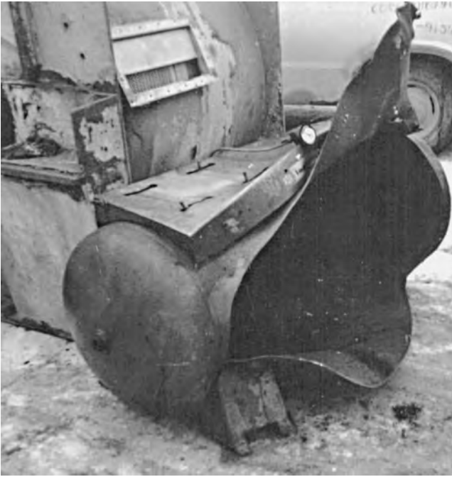
Figure 1.5 An air receiver tank explosion.
