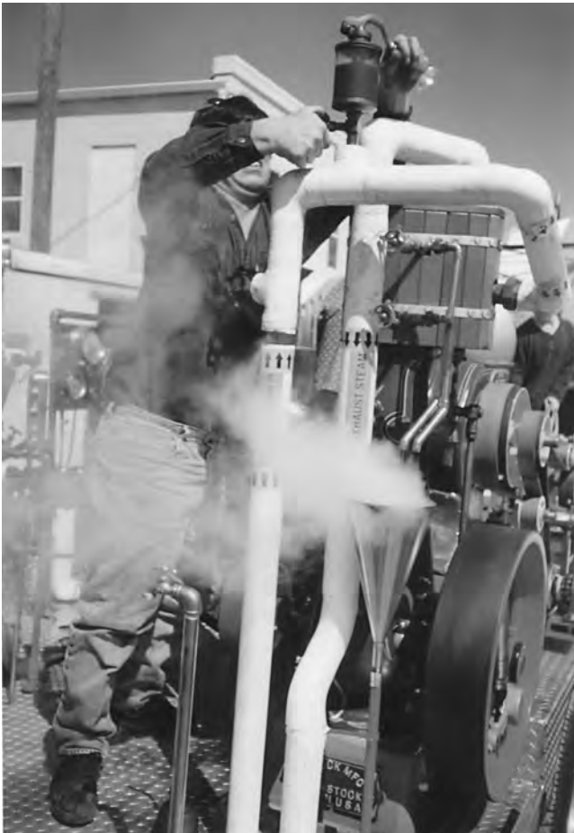
Figure 16.3 Hand lift testing of safety valve by an operator.
