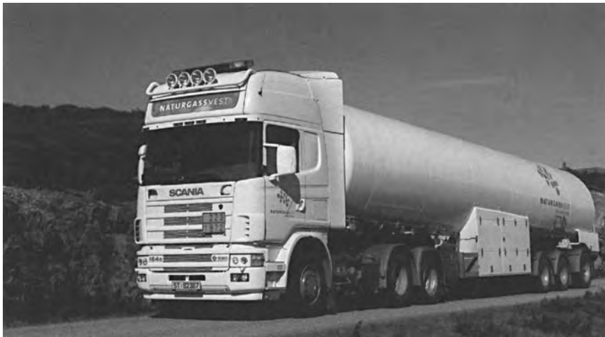
Figure 13.1 A trailer tank for transporting liquefied natural gas. (Courtesy Chart-Ferox, Germany.)
